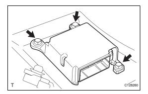
(b) Remove 3 bolts and the center airbag sensor assembly.
